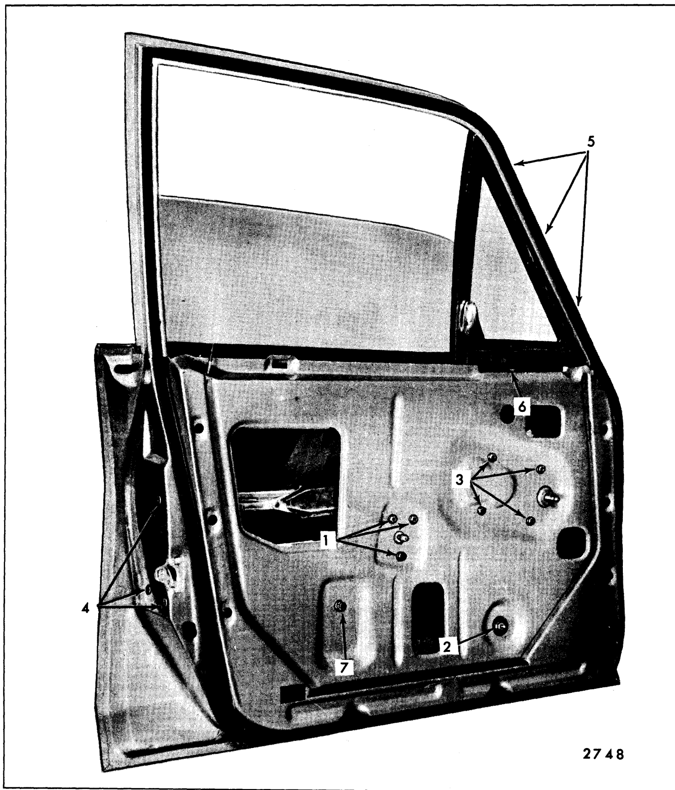
Fig. 6-56—Front Door Hardware - "X-69" Style Shown, "X-27" Style Similar
