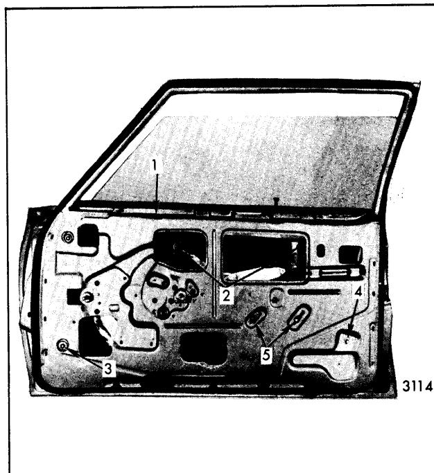
Fig. 6-85—Front Door Window Removal and Adjustment - "B-11" Styles
